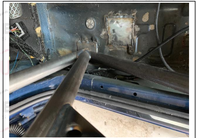
PHOTO 6 FRONT ROLLBAR TO FLOOR ATTACHMENT
