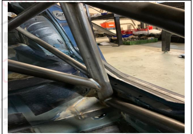
PHOTO 4 MAIN ROLLBAR TO FLOOR ATTACHMENT
